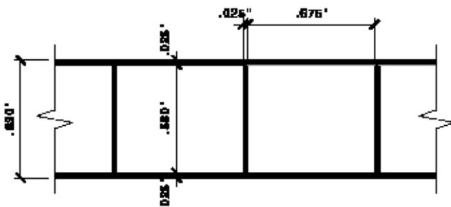
**PANEL SIZES AND TOLERANCES** offered in 4' x 8' (1.2 m x 2.4 m) and 4' x 10' (1.2 m x 3 m). C3 colors are offered in 4' x 8' (1.2 m x 2.4 m) only. Custom sizes and gauges are also available (extended lead time will apply). All dimensions and squareness (standard or custom) are subject to a +/- 1/8" (3.1 mm) cut tolerance.
