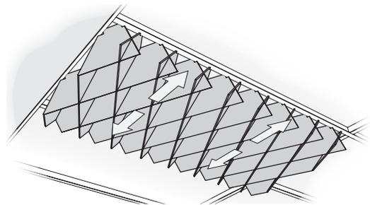
Repeat on the last side with same installation technique. Orient additional baffles in the same direction.
