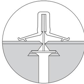
After installing two adjacent Clario Ceiling Baffles, reach up above the grid through an adjoining open space (where a baffle has not been placed yet) and place the clip on the cross tee to keep the Clario Ceiling Baffle in place.
