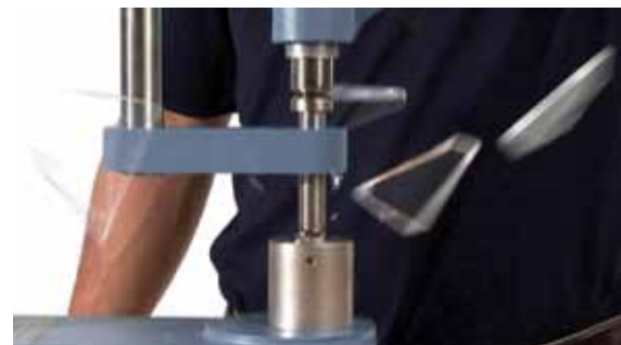
FAILED IMPACT TEST WITH GLASS USING STEEL DART WITH ONE INCH DIAMETER TIP
